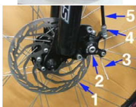
cable sheath (5) brake disc (1) brake caliper (2) brake cable (3) brake adjuster (4)
